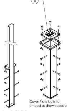
Bolt down Post & Plate assembly to embed
